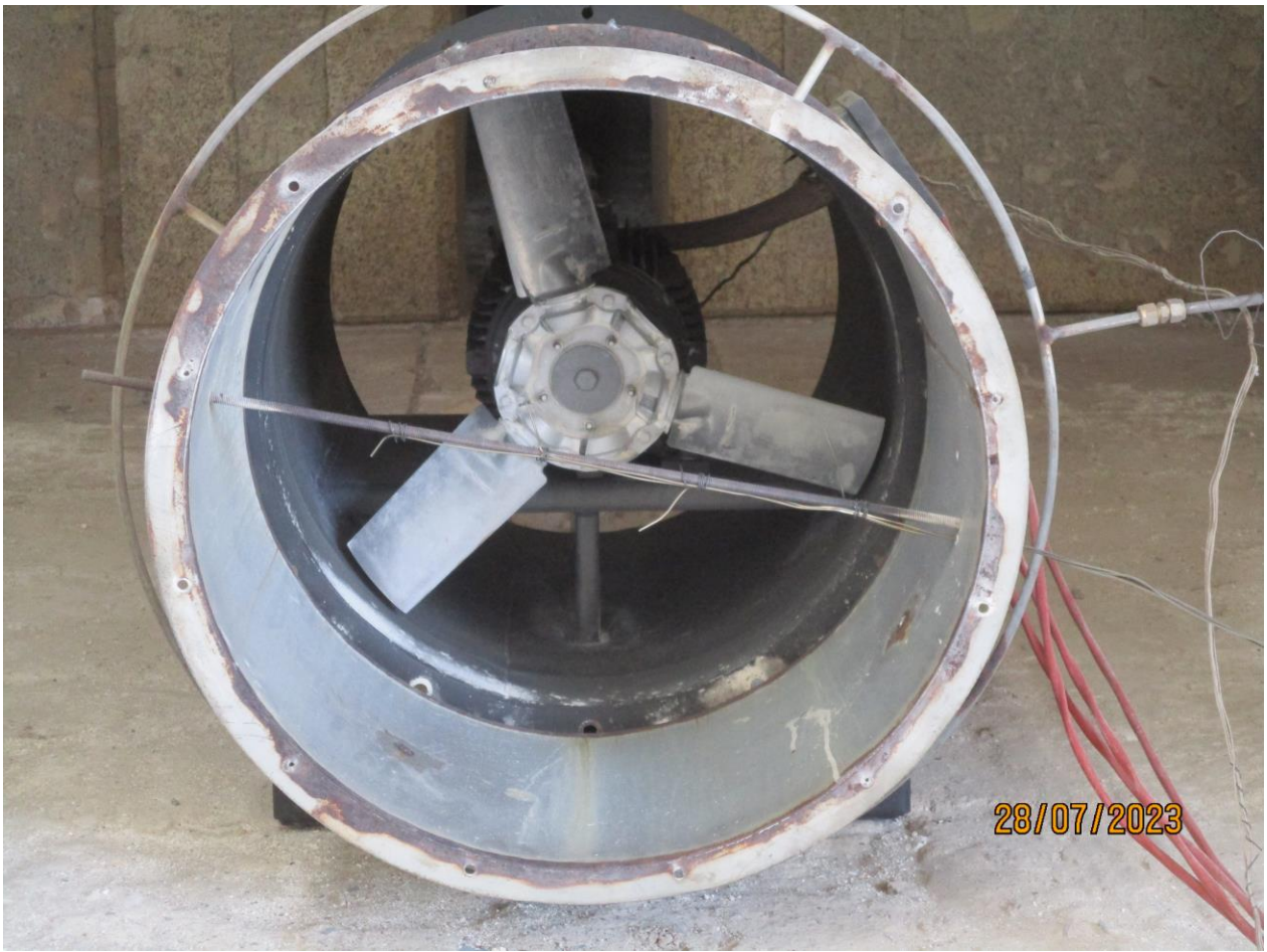
Photo C3: Front view of the specimen after the test
